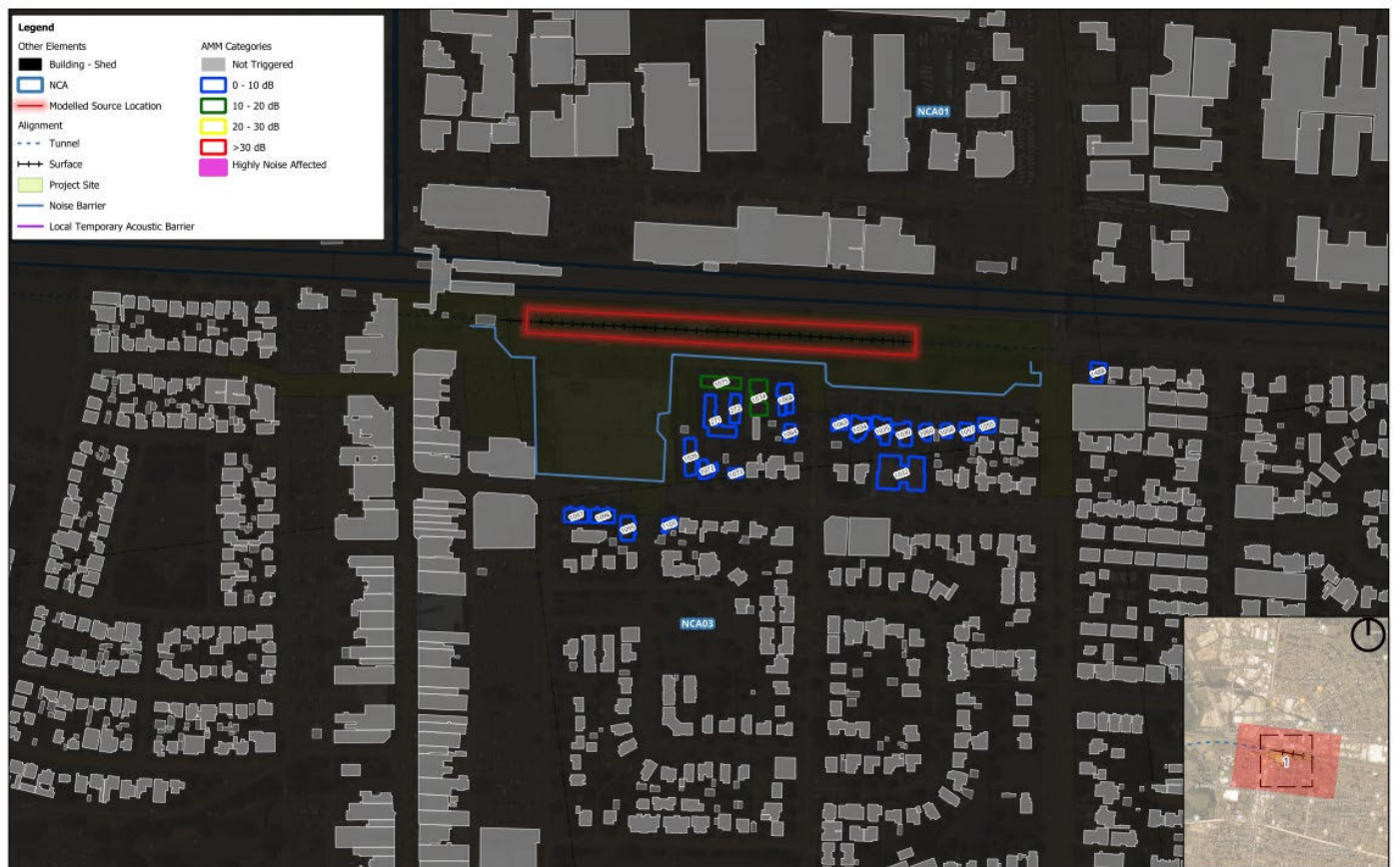
FIGURE 5. CONCRETE FINISHING WORKS NOISE MODELLING MAP SHOWING PROPERTIES CONSULTED WITH IN THE 10 – 20 DD AMM
