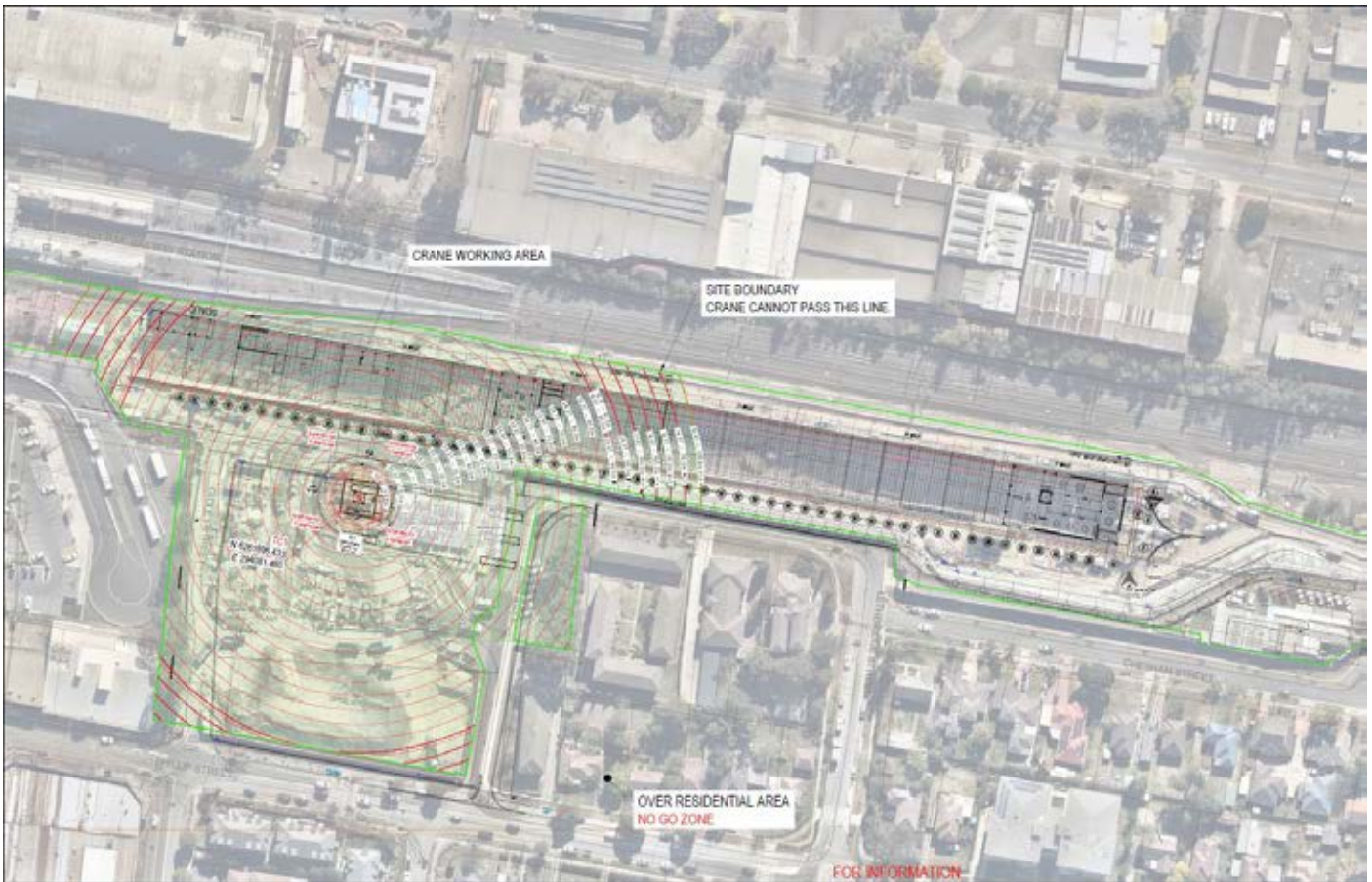
FIGURE 17: TOWER CRANE 1 LOCATION
