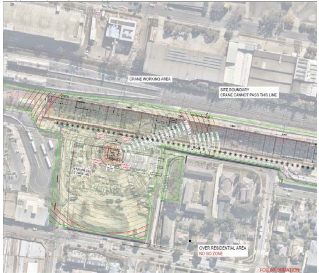
FIGURE 1: TOWER CRANE 1 LOCATION
