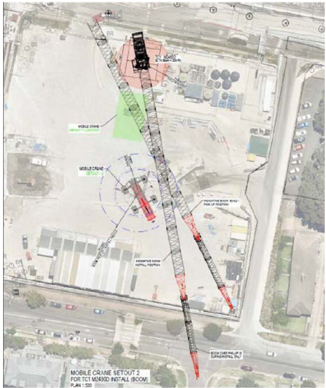
FIGURE 4: SET UP FOR INSTALLATION OF BOOM, MAIN HOOK AND FLY HOOK FOR TOWER CRANE 1
